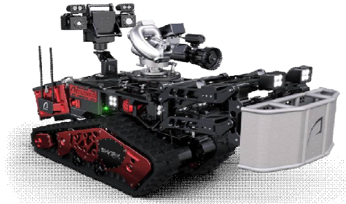
Figure-Shark Robotics Fire Extinguishing Robot
